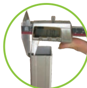
Use 1.7mm thick aluminium in legs
